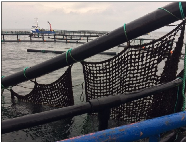
Picture 2: The set up with two nets with different mesh sizes alongside each other on a 10 meter PVC tube.
