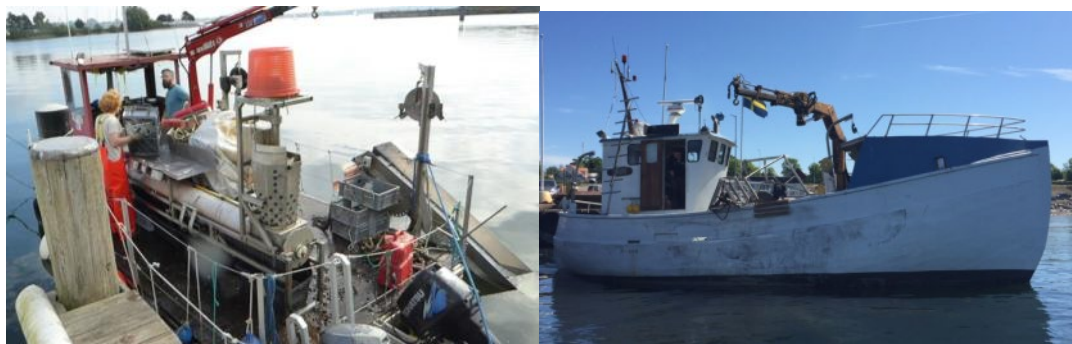
Figure 30. Left: Pontylus, the work platform used at the Kiel farm. This type of platform works at protected sites but could not be used in open water. Right: The fishing boat used as work vessel at the Byxelkrok farm. This is an example of boat not suitable for mussel farming. It did not act as a stable platform during anchor drilling or when attached to the mussel farm, so the work could only be done in calm days.
