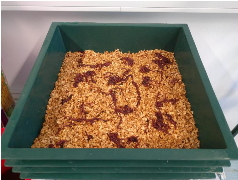
Picture 5: Vermifiltration unit stocked with worms prior to the first feeding.
