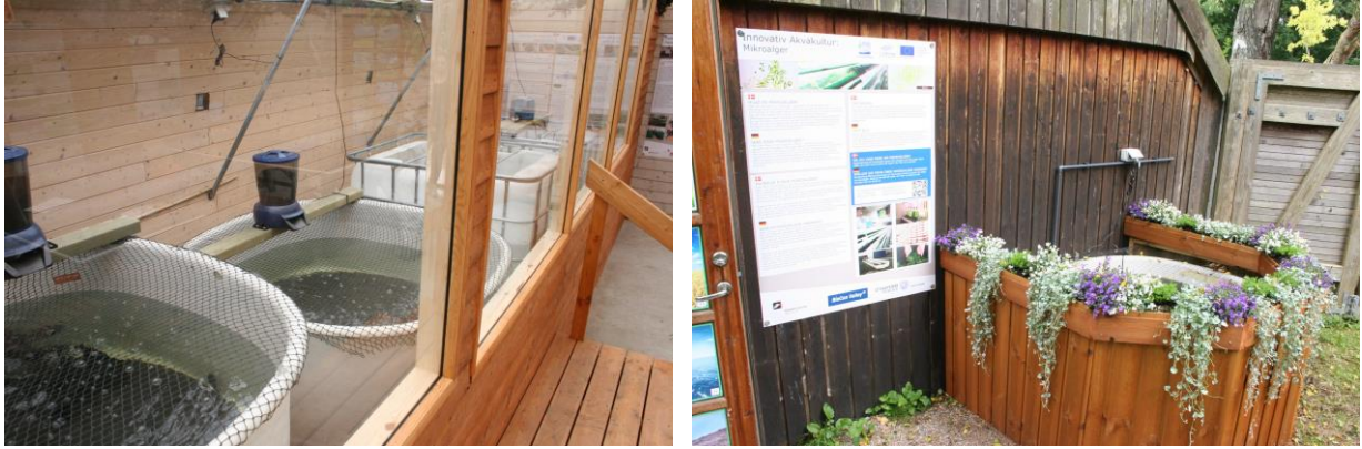
Picture 1: The pilot RAS facility at Guldborgsund Zoo (the fish tanks, including automated feeders in front and the water treatment in the back.
